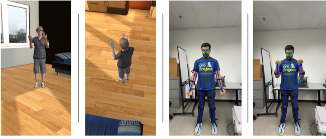
Fig. 5. Comparison between camera-based pose estimation and 3D avatar-based motion visualization for biceps curl tracking. The figure illustrates the limitation of single-view camera-based pose estimation, which provides joint angles from a fixed 2D perspective, compared to the proposed 3D virtual environment where the avatar can be observed from multiple viewpoints. This enables more comprehensive analysis of arm movement and joint angles during biceps curl exercises.
